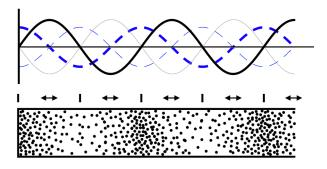
The thick blue dashed line shows the pressure distribution along the tube at this instant while the thick black curve shows the speed.
