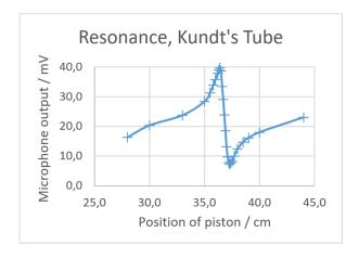
The sudden change in sound pressure can be heard as well as measured and can be used to quickly find the vicinity of the nodes. For the final fine tuning of the piston, use only the microphone voltage – not your ear.
