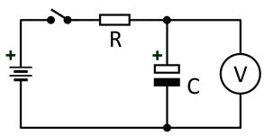
In the schematics, the power supply is drawn as a battery.
