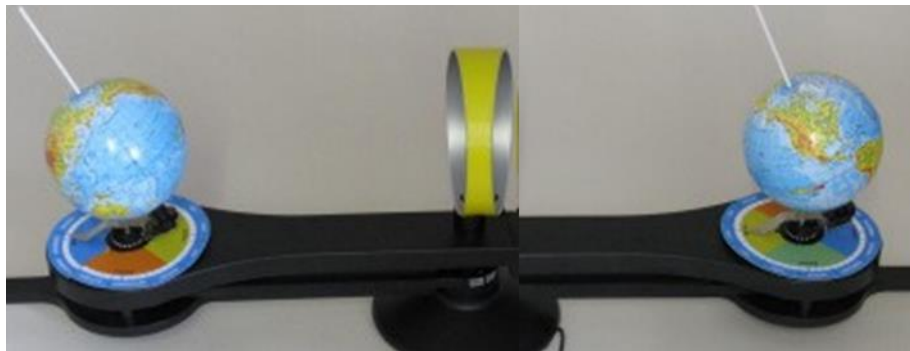
Fig. 5 The Earth's axis pointing 'up and left' creates a Northern Hemisphere summer (right) and, six months later on the opposite side of the Sun, winter (left). The season and date are indicated by the position of the pointer over the date disc.
