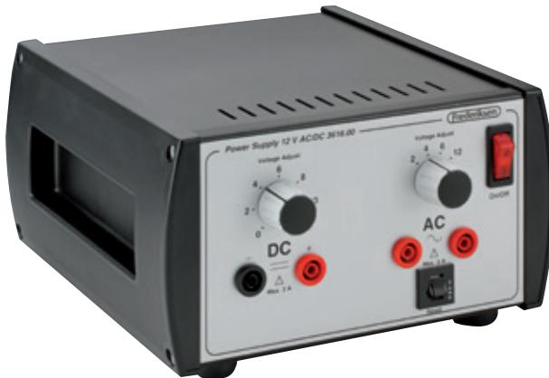
The power supply delivers a stabilized DC voltage, continuously adjustable between 0 and 12 V. Moreover, an AC voltage is supplied, which can be set to 2, 4, 6 or 12 V. The AC voltage is not stabilized.
